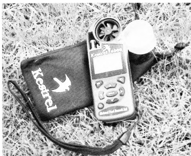
Fig. 2. The Kestrel 4000 has its own carrying bag. The protector for the impeller on the anemometer is open in this picture. The device is clearly very portable.
