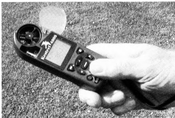
Fig. 1. Taking a temperature reading. The store rate of the data log can be set to anywhere between 2 seconds and 12 hours. It continues to take readings even when the device is switched off. It is a bit like having a 'Black Box' in your pocket.
