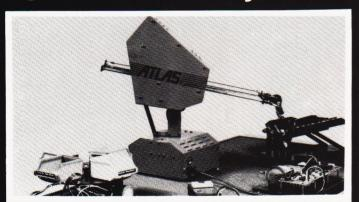
Based around the popular LJ ATLAS Robot, this work-cell provides an automatic parts-selection system running under full microcomputer control.
