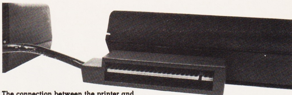
The connection between the printer and the ZX81 allows the RAM Pack to be attached at the same time, as seen in the picture at the foot of this page.
