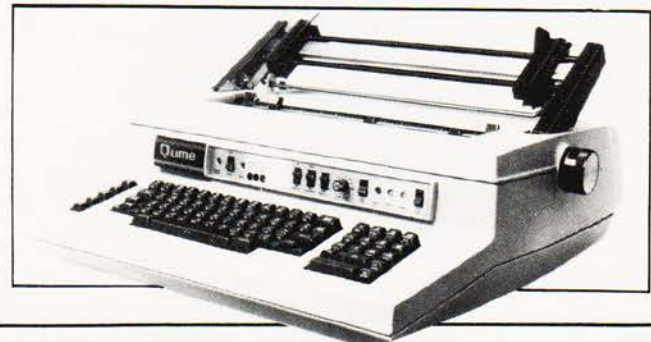
The Qume Spirit 5 Daisy wheel printer.
