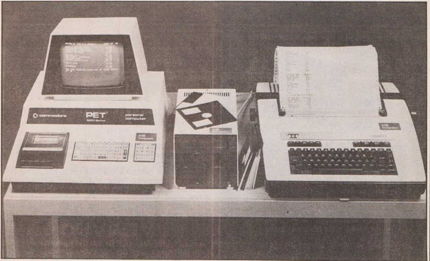
A view of a typical small business, or advanced home computer, system. The PET has had the expansion memory fitted to hold the operating system. The printer is connected to the PET via an adaptor, IEEE-488 to RS232, for system output.
