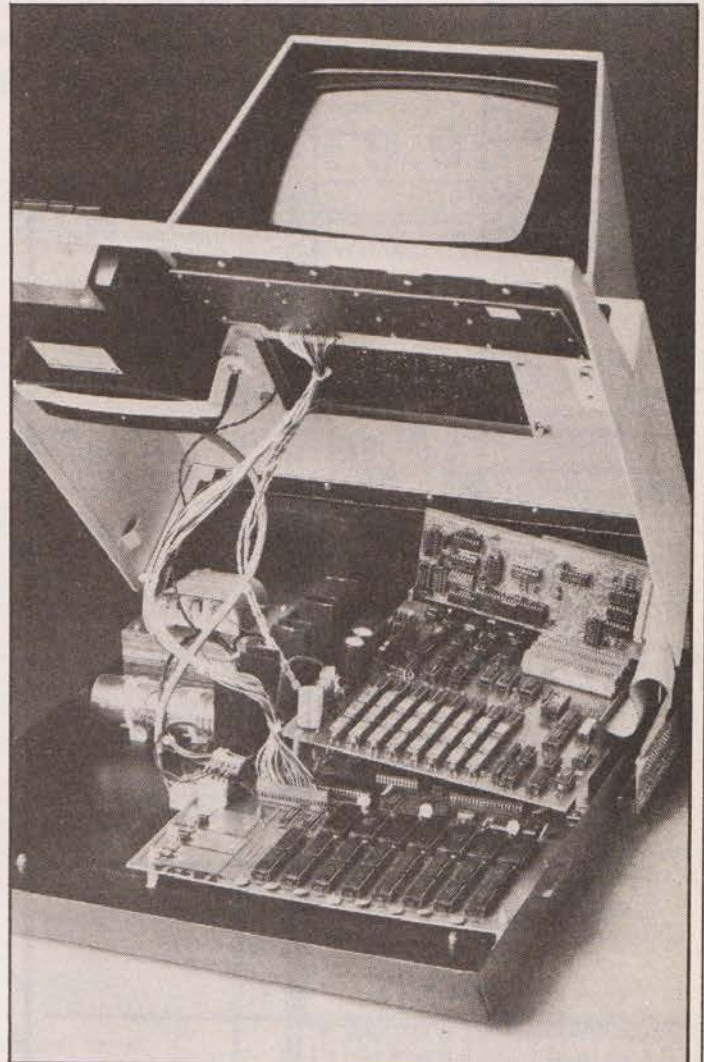
The sloping board with the vertically aligned daughter boards is the ExpandaPET memory which is essential for the operation of the disk system.
