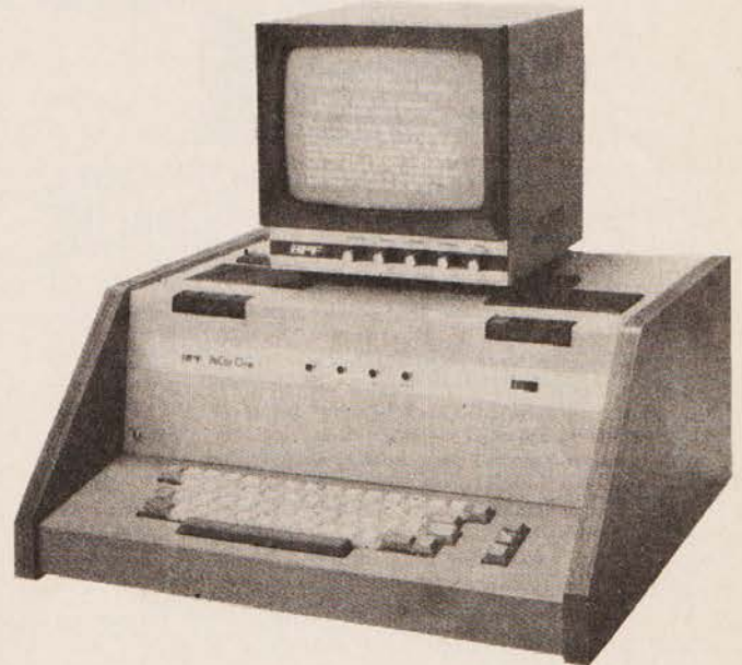
The PeCos One which is made in the Far East for a US customer. It includes 24K ROM and 16K RAM.
