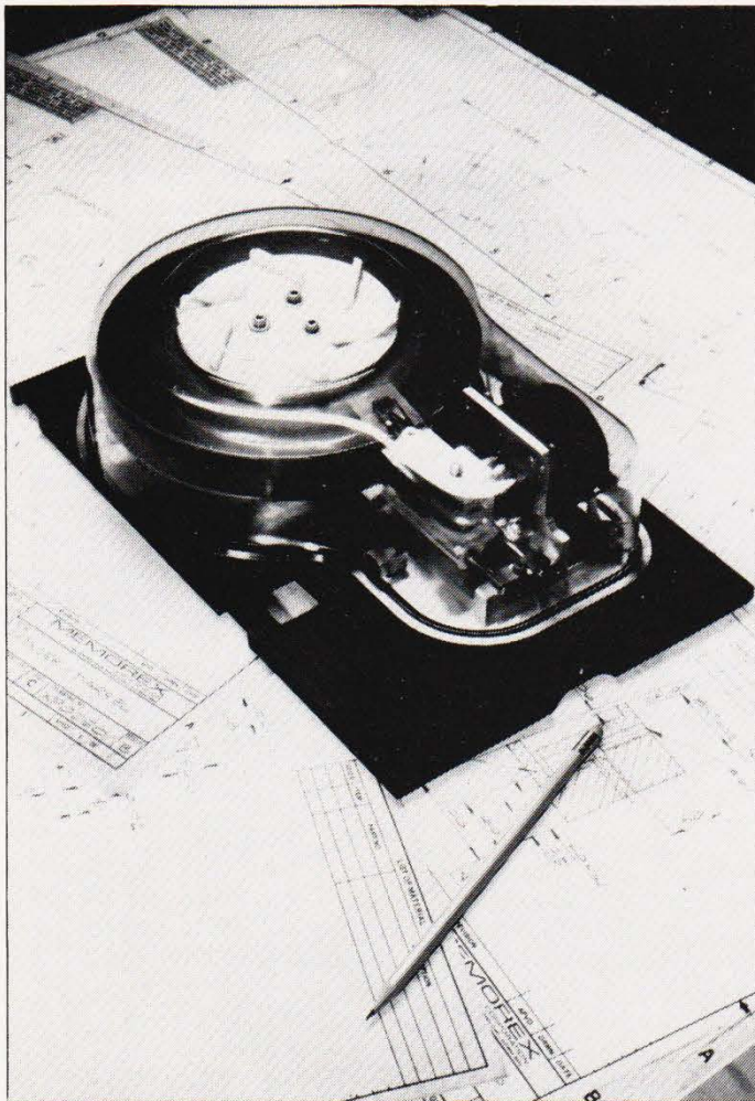
This Memorex Winchester uses dual platters to give 11.7 Mbytes of store.
