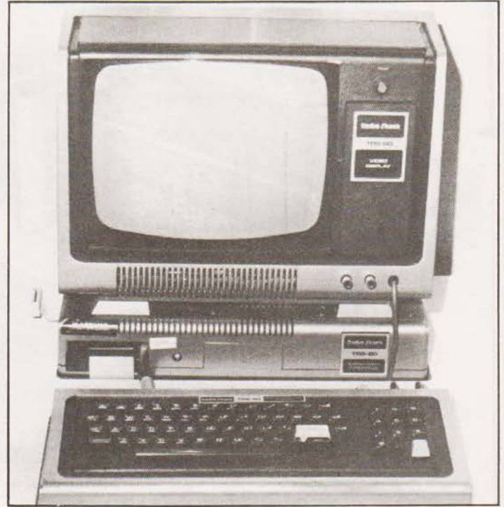
The debated TRS 80 monitor. If you modify the modulator circuit as shown below you can use your telly instead and save yourself a few pennies.
