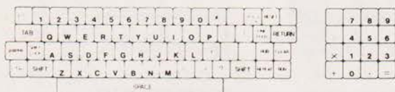
Figure 4. Characters with Shift Lock Key Depressed
